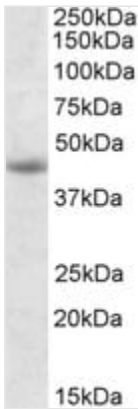
WB (Western Blot) 1ug/ml staining of Jurkat lysate (35ug protein in RIPA buffer). Primary incubation was 1 hour. Detected by chemiluminescence.
