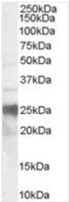
WB (Western Blot) 0.3ug/ml staining of Human Brain lysate (35ug protein in RIPA buffer). Primary incubation was 1 hour. Detected by chemiluminescence.
